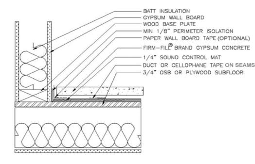
When installing sheet vinyl and vinyl composition tiles over FIRM-FILL® Gypsum Concretes, in all cases, floor covering manufacturer recommendations supercede these guidelines.
